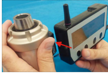
Fig. 13b. Slide transmitter across 'detection side' of the display
