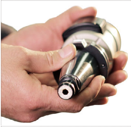
Fig. 30. Example of toolholder with a coolant-through hole
