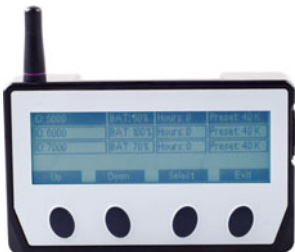
Fig. 21. Disconnection list on Multiple Signal screen
