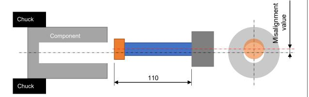
Pre hole dia. : φ15.8 Finish hole dia. : φ16 Misalignment value : 0.3mm
