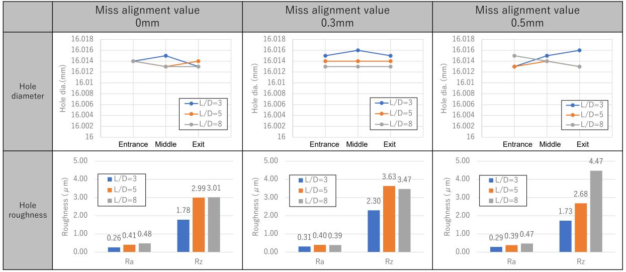
Hole diameter: Regardless of the L/D ratio or miss alignment value, ReamMeister can get consistent hole diameter within H7 tolerance. Hole roughness: While there is a tendency for the surface roughness to worsen as the L/D ratio and miss alignment value becomes bigger, overall, ReamMeister offers satisfying roughness.
