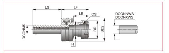
XThe holder side can be adjusted up to maximum of 1.6mm, but it cannot adjust an offset beyond the radial cutting edge length on the reamer.
