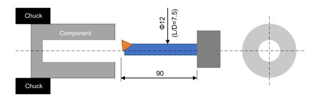
Pre hole dia.  $: \varphi 15$ Finish hole dia.  $: \varphi 16$
