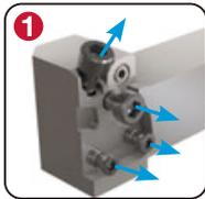
**1** Remove all 4 screws and ensure the O rings are all in place.
