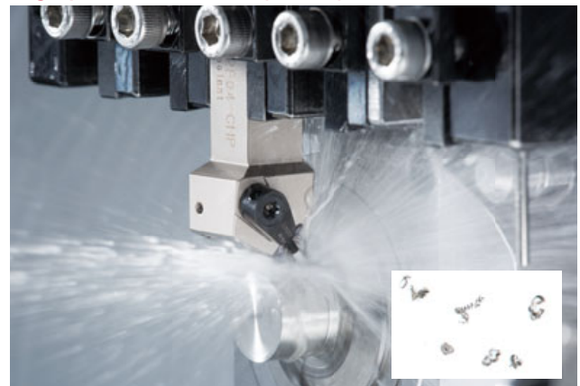
High pressure coolant (7 MPa)
