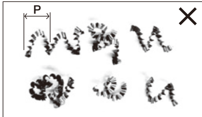
Continuously curled "C" shape chips with short lead (P).
