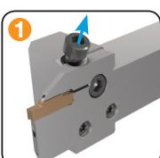
First loosen the long screw in the angular direction.
