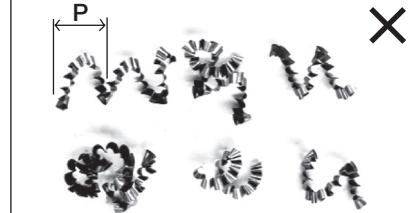
Continuously curled "C" shape chips with short lead (P).
