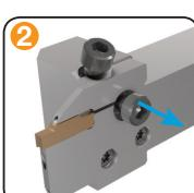
Loosen the Fixing screw in the center and remove the insert.
