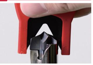
Tighten by a clockwise twist
