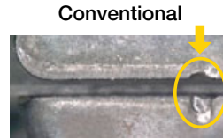
Edge fracture occurred due to low cutting edge strength
