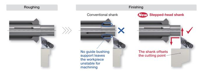
Prevents chips from entering the guide bushing during thread machining.
