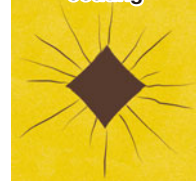
Indentation test on coating
