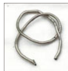
送り: f = 0.025 mm/rev 切込み: ap = 2 mm
