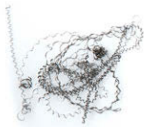
External coolant supply (at normal pressure)
