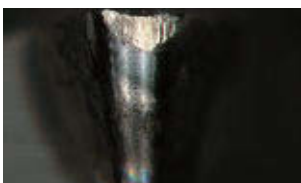
External coolant supply (at normal pressure)
