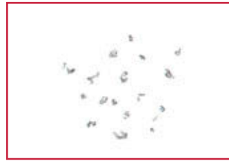
High pressure coolant (>7MPa)
