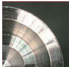
TETRAMCUT Good surface finish with no chatter marks
