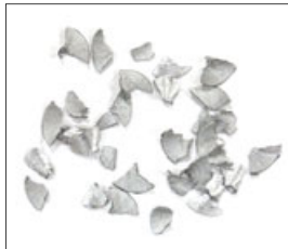
Aluminium alloy casting (ADC12)
