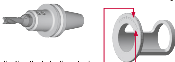
Scale for adjusting the hole diameter in milling machine (Periphery of sleeve)
