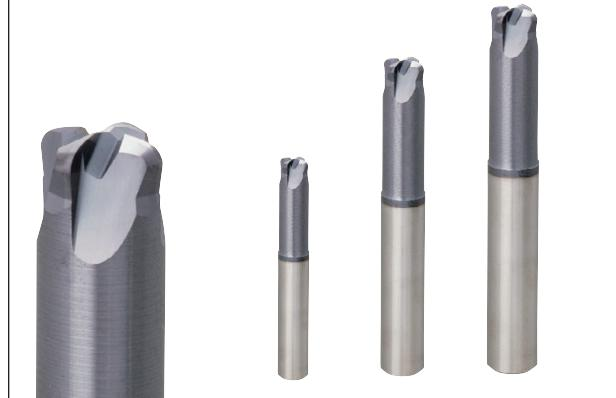
Due to this geometry, the solid **FeedMeister** can operate at feed per tooth (*fz*) rates up to 0.5 mm/z, at 0.3 to 0.7 mm depth of cut (*ap*), providing a significant reduction in cycle time, which thus increases productivity.
