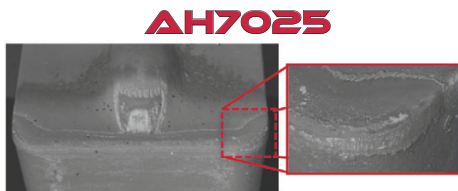
Tool wear after 60 grooves
