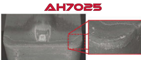
Tool wear after 60 grooves
