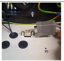
Carefully lay the device on its back and connect the plug of the scanner cable. Secure the cable with the cable glands.
