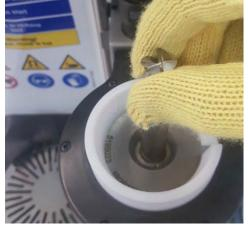
Insert the tool into the tool holder or remove the tool that has already been inserted.
