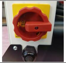
Connect the power supply using the CEE-CEKON connector.
