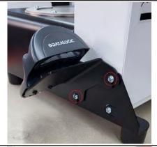
Loosen the two marked screws untill scanner holders plate slots can accomodate them.
