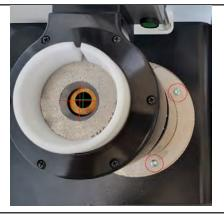
If inserted stop disc is no concentric with the tool holder, the shrink position can be fine-tuned. Minor errors can be compensated by loosening the screws marked on the picture and then readjusting crescent-shaped positioning plate
