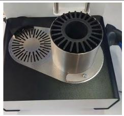
Place the appropriate tool holder in the shrink position under the coil.
