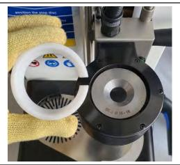
Remove the clamping ring by manually pressing and a pole disc that may already be inserted. Insert the appropriate pole disc for the tool holder and the tool into the coil and secure it again with the clamping ring. Move the coil to the top end position.
