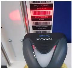
Use the handheld scanner to scan the appropriate barcode for the tool holder to set the operating parameters for the next shrink operation.
