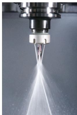
With angular four nozzles. Coolant flow is direct to the cutting edge - for use with standard straight shank cutting tools (without coolant hole).
