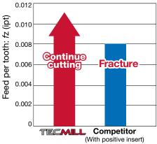
Work material : 1055 (200HB) Tool ø :  $\emptyset$ 2.000" Cutting speed : Vc = 820 sfm Depth of cut : ap = 0.118" Width of cut : ae = 0.500"
