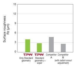
With standard inserts only and no wiper, TPW provided better surface roughness compared to Competitor A with no radial run-out adjustments. With standard + wiper inserts mixed, TPW provided the same surface quality as the competitor B with radial run-out adjustments.
