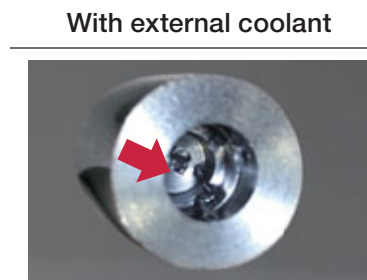
Chip not completely removed, causing damages to parts
