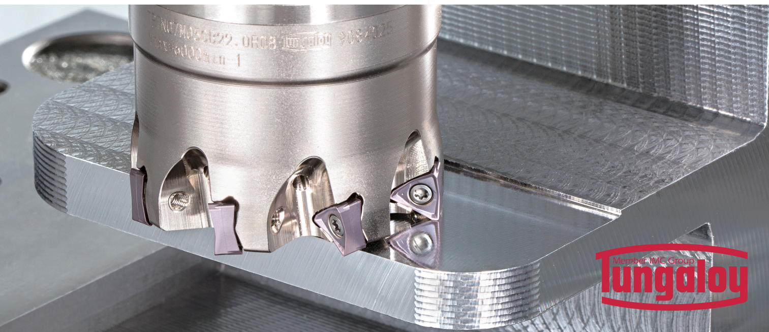
TN MU07-MJ with built-in wipers APMX = 0.256"
